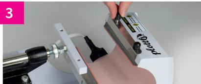
3 Tip: When inserting a new attachment, make sure that you mount it with both screws on the left side first.
