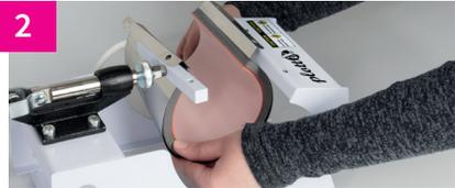
2 Pull the lever backwards to open the press and remove the attachment from the metal rack.
